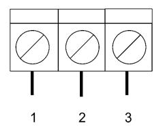
Pins 1 & 2 are connected to sensors same pin. User shall wire terminals 2 & 3 in case of 2-wire connection.
