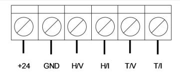
+24: +24Vdc power supply GND: power supply ground HV: 1...10Vdc output for 0...100% r.h. humidity HI: 4...20mA output for 0...100% r.h. humidity TV: 1...10Vdc output for temperature (consider scale table) TI: 4...20mA output for temperature (consider scale table)
