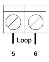
The sensor is not polarity sensitive. Avoid applying voltages greater than 30VDC.
